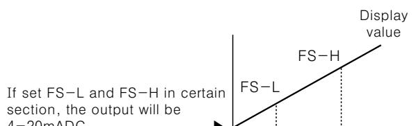
When the resolution is 8,000 division from FS-L to FS-H, the resolution will be lower when the display value is narrower than 8,000 division.
